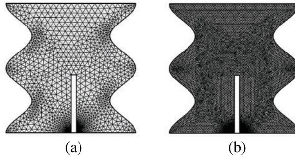
**Figure 2:** Distribution of the grid size of (a) 1702 and (b) 13273 elements
