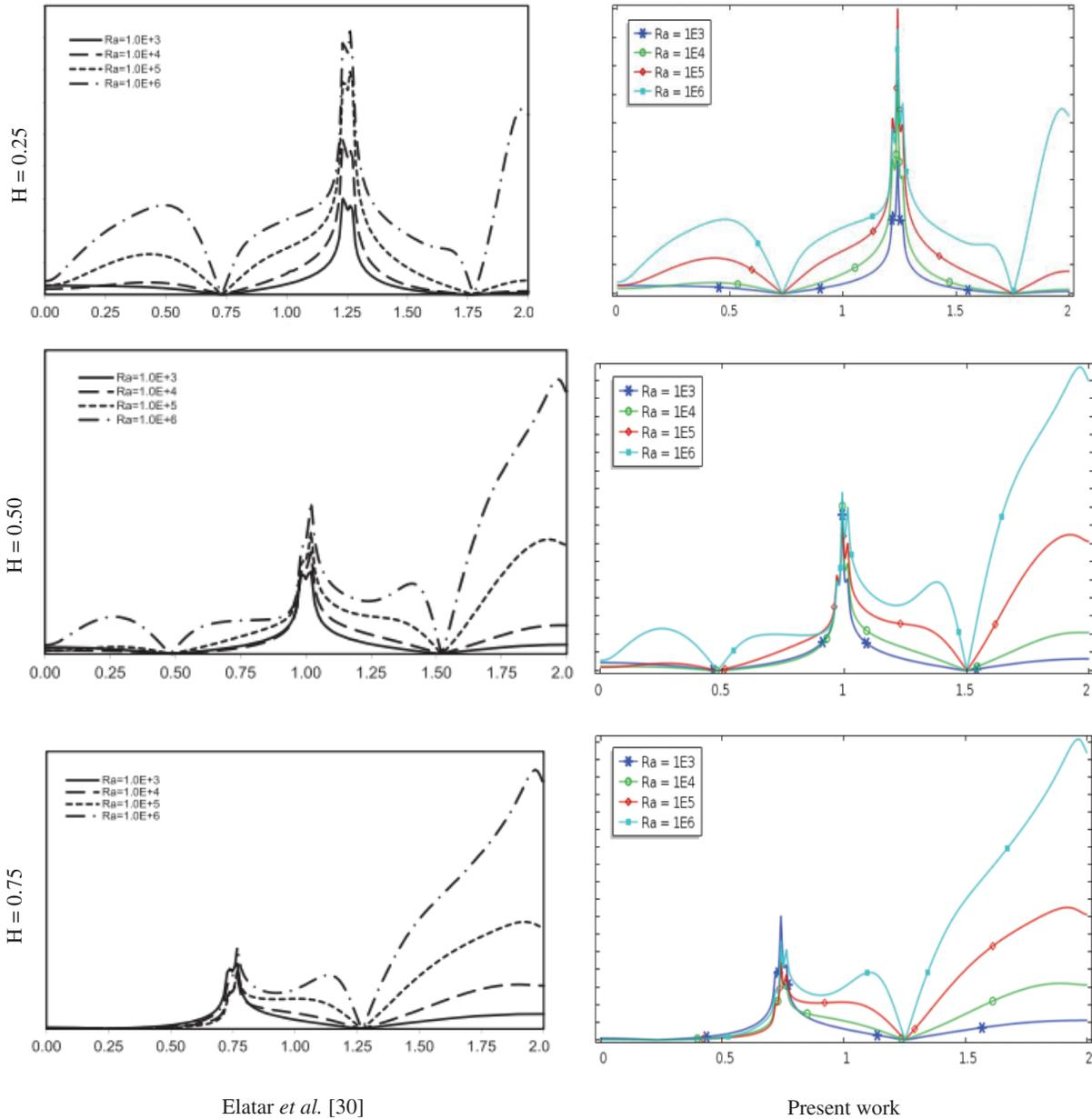
**Figure 4:** Comparison of  $Nu_L$  variant  $H$  and  $Ra$  at  $L = 0.5$  and  $B = 0.01$
