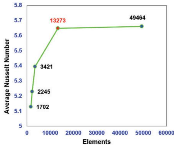
**Figure 3:** Grid survey for several elements
