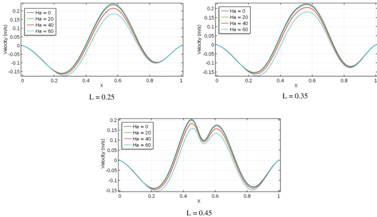
**Figure 7:** Velocity sketches for different  $L$  and  $Ha$  at  $A = 0.10$ ,  $\lambda = 2.0$  and  $Ri = 1.0$
