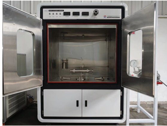
Figure 3: Core flooding apparatus
