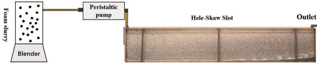
Figure 2: Dynamic sand-carrying device
