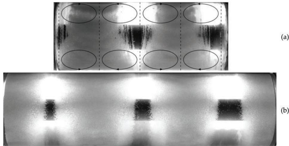
**Figure 3:** Photos of granular medium and liquid obtained (a) in the short cavity #1 ( $f_r = 4$  rps,  $f_{osc} = 1$  Hz,  $\varepsilon = 0.36$ ) and (b) in the long cavity #2 ( $f_r = 4$  rps,  $f_{osc} = 1.82$  Hz,  $\varepsilon = 0.45$ ). The dashed lines indicate the location of pressure antinodes. The vertical pairs of ellipses illustrate the cross-section of the vortices (arrows show the direction of steady rotation)
