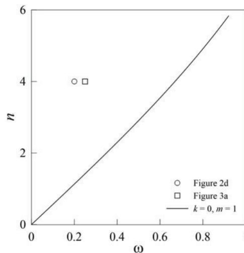
**Figure 4:** Dependence of axial wavenumber on dimensionless frequency. The results of the calculations (solid line) and experiments (symbols) correspond to cavity #1
