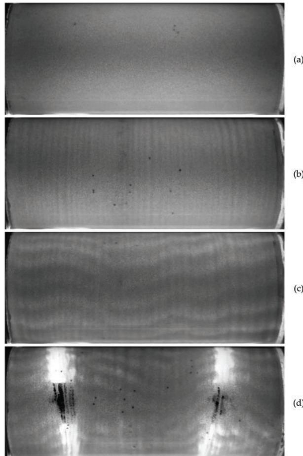
**Figure 2:** Photos of granular medium and liquid obtained at rotation rate  $f_r = 5$  rps and oscillation frequency  $f_{osc} = 1$  Hz in the cavity #1 (a–d):  $\varepsilon = 0, 0.17, 0.24,$  and  $0.32$ . The black horizontal band in photo (d) is the inner boundary of the cylindrical annulus which is formed by a black-painted metal tube
