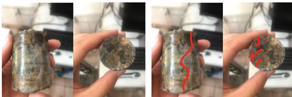
Figure 10: Physical image of No. 8 core after water flooding
