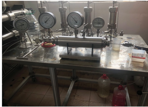
Figure 1: Water sensitivity test device of conglomerate cores
