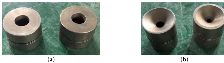
Figure 5: Jet pump partial structure diagram: (a) physical diagram of the diffuser section; (b) physical diagram of the throat section.
