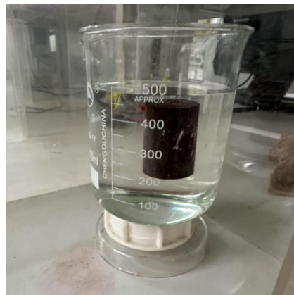
Figure 3: Physical experiment diagram of core imbibition experiment.
