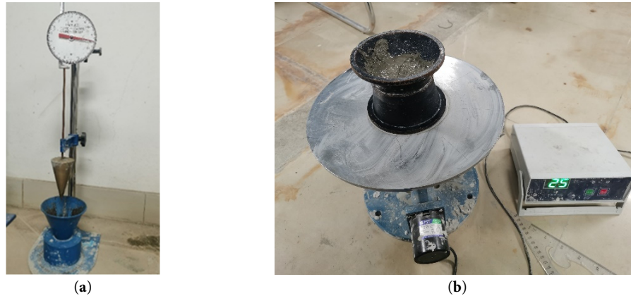
Figure 1: Slurry fluidity test apparatus: (a) Consistency tester; (b) Jumping cone method collapse degree tester.
