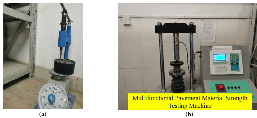
Figure 3: Slurry strength test apparatus: (a) Solidification time tester; (b) Cubic compressive strength tester.
