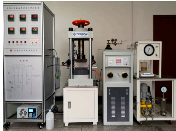
Figure 1: Fracture flow conductivity testing apparatus.
