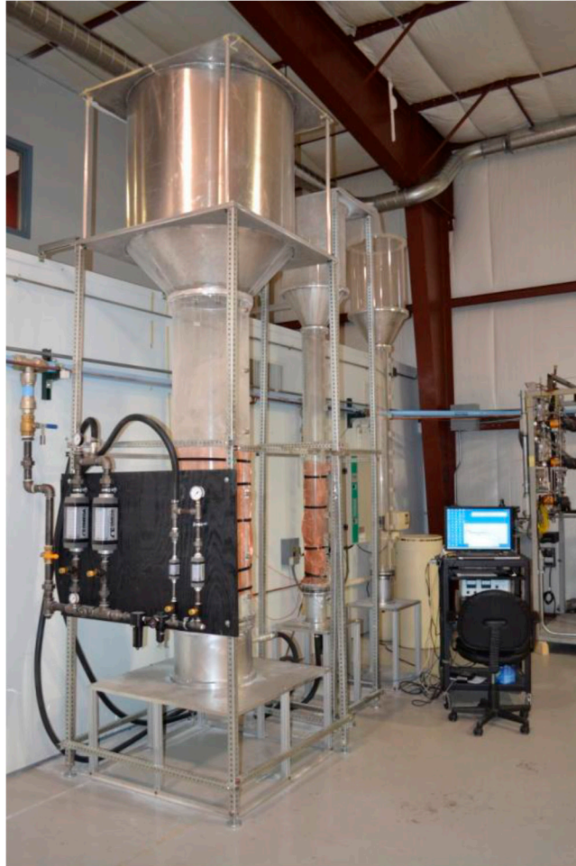
Figure 2: A photograph of the large and small scale gas-solids fluidized beds used in this study, along with the air flow system that was utilized [30].
