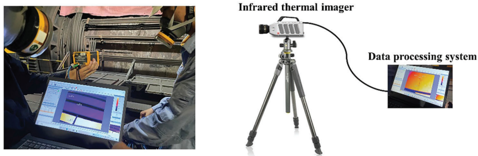
Figure 4: Schematic diagram of temperature monitoring
