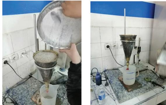
**Figure 7:** Manipulation of Marsh cone on the plaster paste incorporated by JM fibers
