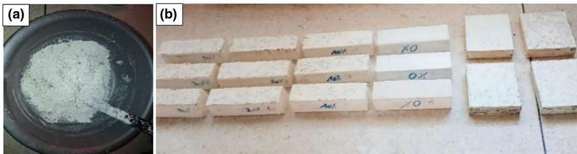
**Figure 6:** (a) Mixing of fibers with plaster, (b) shapes of demolded composites
