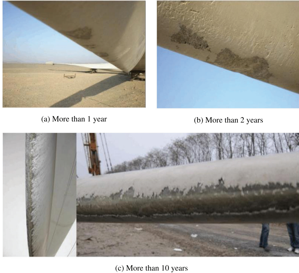
Figure 2: Erosion of blades according to service life
