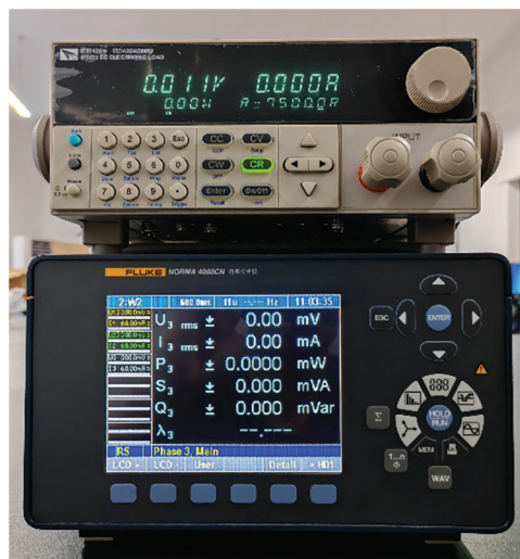
Figure 5: Aerodynamic characteristics and noise measurement process with related equipment: power analyzer type NORMA 4000CN and electronic load meter type IT8512A+
