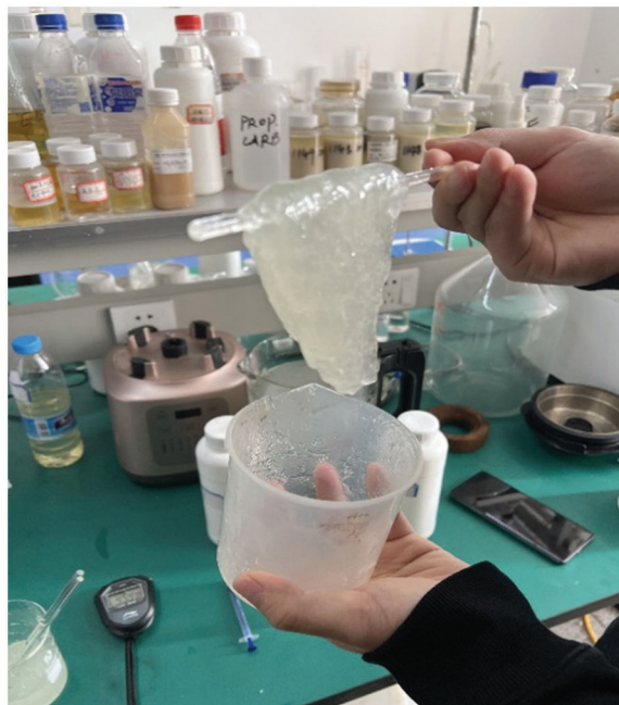
Figure 6: Morphology of crosslinked fracturing fluid
