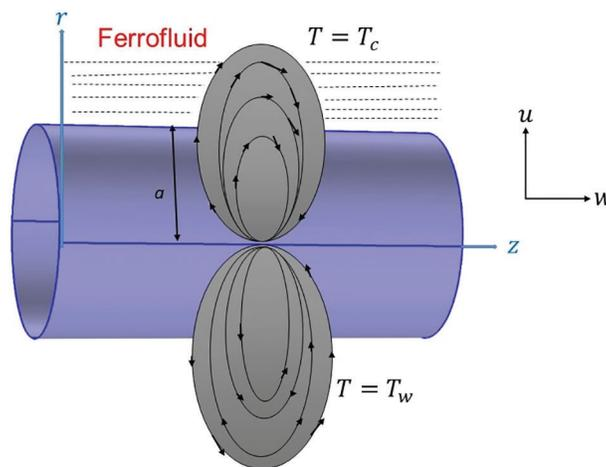
**Figure 1:** Ferrofluid flow layout over a stretched cylinder upon the existence of a permanent dipole
