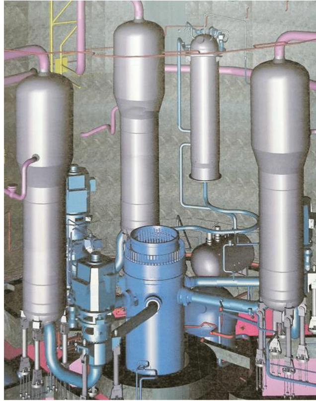
Figure 1: The primary loop of the HPR1000
