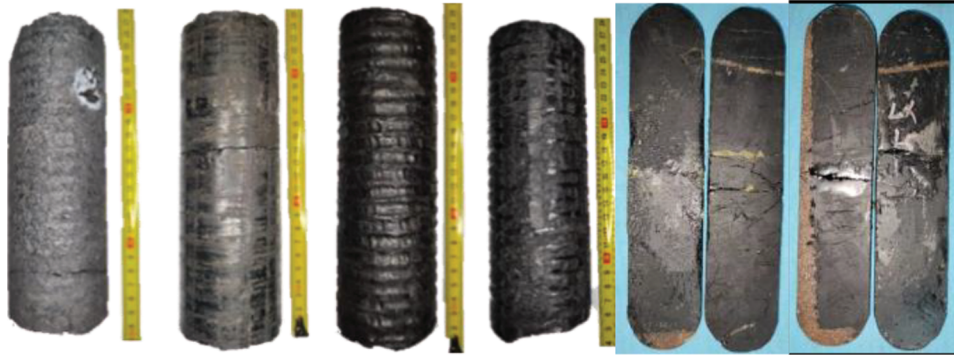
Figure 3: The core and coal rock slab in Linxing-Shenfu block of deep coal fracture
