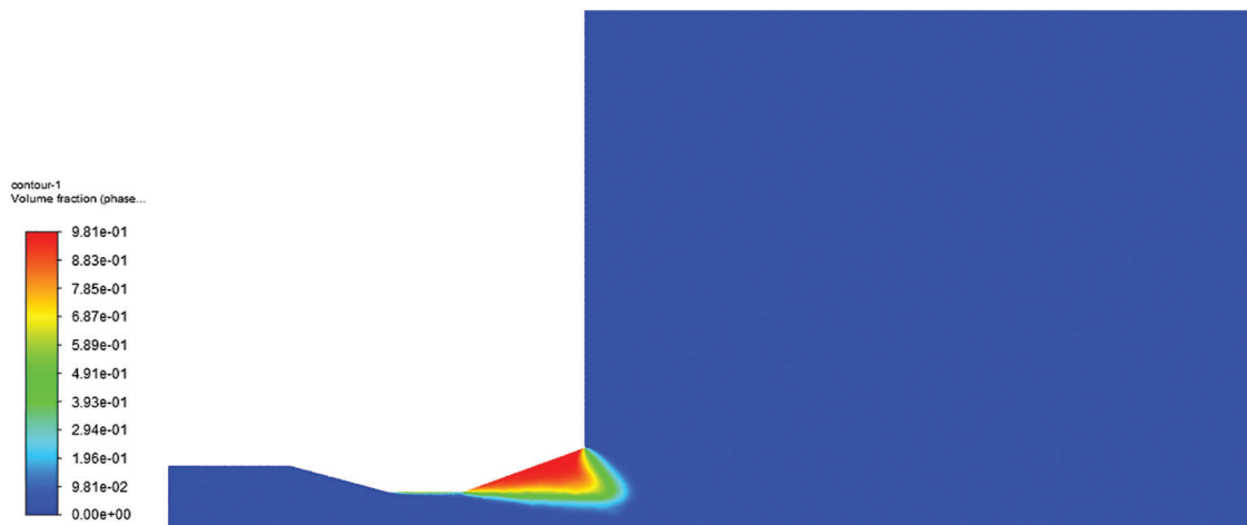
Figure 7: Flow field gas volume fraction contour
