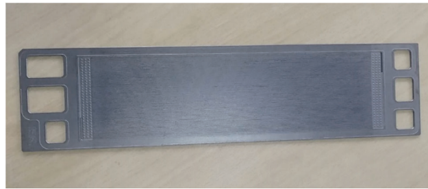
Figure 3: Graphite bipolar plate in test
