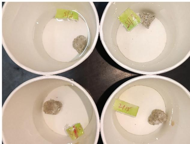
**Figure 6:** Mortar specimens for the NMR test
