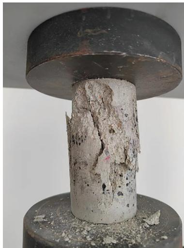
**Figure 5:** Picture of the compressive strength test
