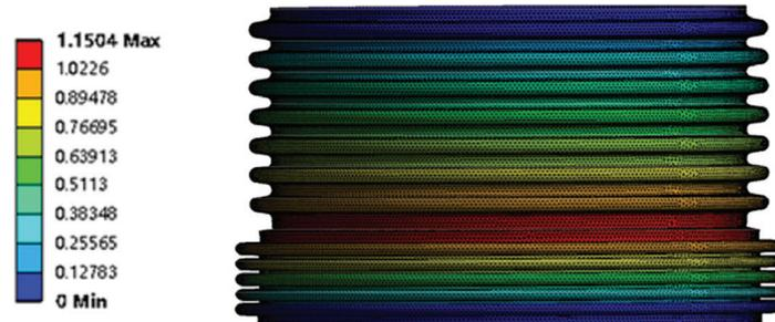
Figure 18: Axial displacement cloud map after deformation
