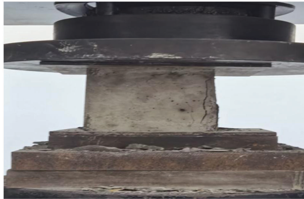
Figure 2: 28-day specimen compressive strength test
