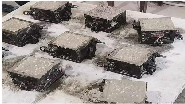
Figure 1: Condition of specimen pounded for 120 s
