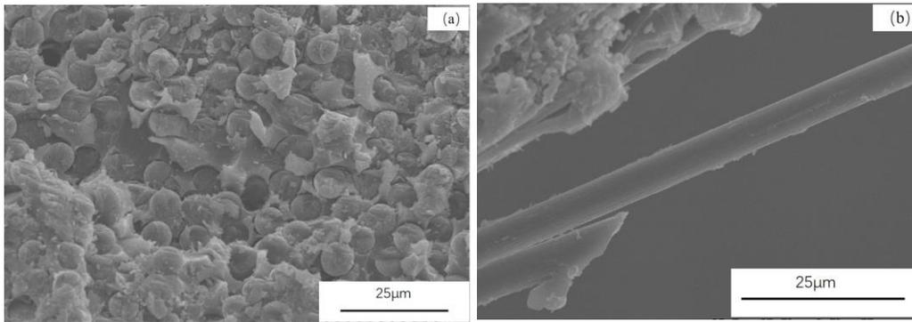
**Figure 8:** SEM images of T800 grade carbon fiber RTM cyanate ester composites
