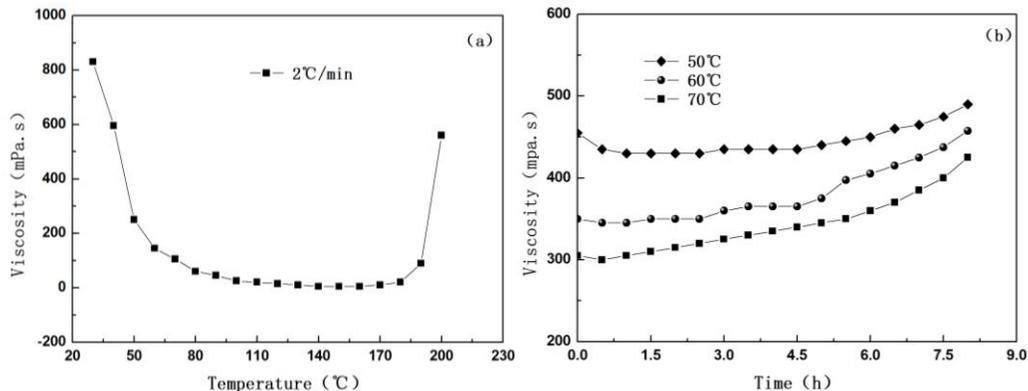
**Figure 1:** Dynamic viscosity (Fig.1(a)) and isothermal viscosity (Fig.1(b)) of cyanate ester
