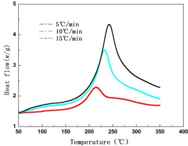
**Figure 2:** DSC curves of cyanate ester for RTM
