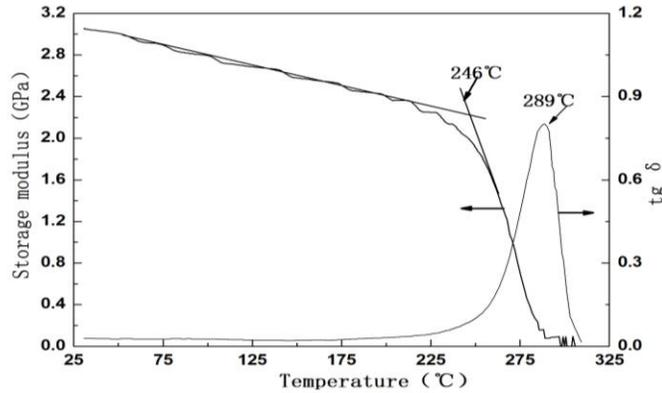
**Figure 6:** DMA curves of cyanate ester for RTM
