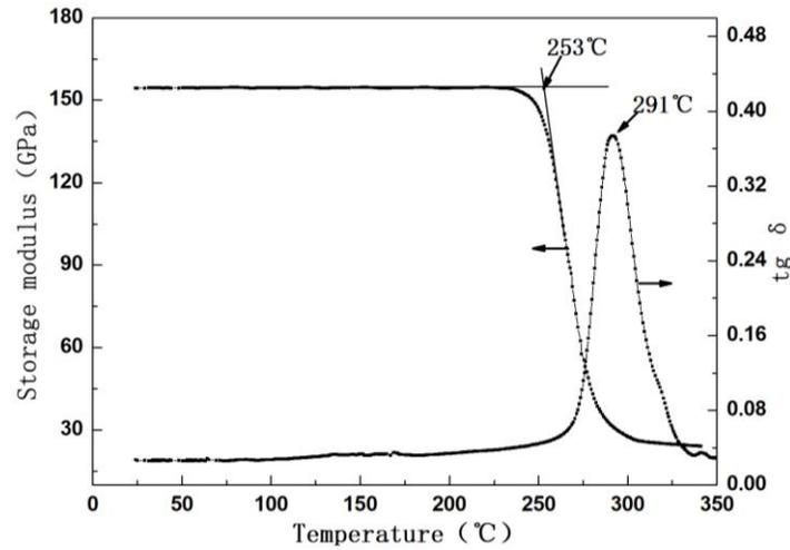
**Figure 7:** DMA curves of T800 grade carbon fiber RTM cyanate ester composite
