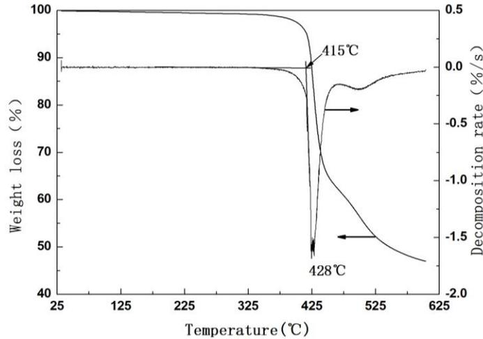
**Figure 5:** TGA curves of cyanate ester for RTM
