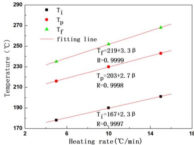
**Figure 3:** Relationship between the characteristic temperatures and the heating rate of cyanate ester
