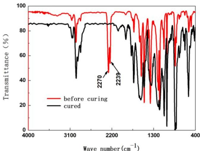
**Figure 4:** FT-IR of cyanate ester for RTM
