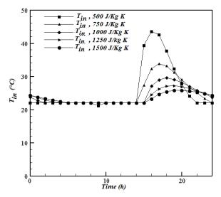
Figure 9.a: Variation of the internal temperature as function of  $c_{p,m}$ .
