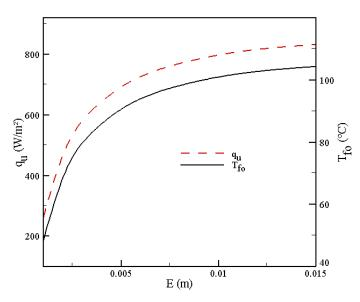
Figure 5.b: Variation of the useful flux and the outlet temperature as a function of the thickness of the absorber at solar noon.
