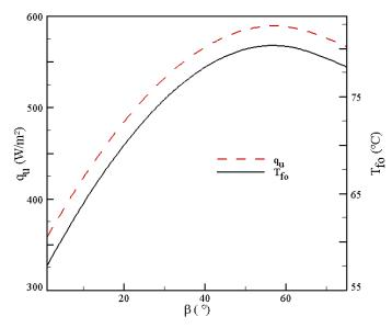
Figure 4.a: Variation of the useful flux and the outlet temperature as functions of the tilt angle at solar noon.
