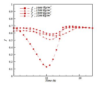
Figure 10.b: Variation of the liquid fraction as function of  $\rho_m$ .
