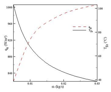
Figure 6.b: Variation of the useful flux and the outlet temperature as a function of the water flow rate at solar noon.
