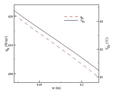
Figure 5.a: Variation of the useful flux and the outlet temperature as a function of the distance between the collector tubes at solar noon.
