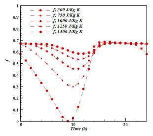
Figure 9.b: Variation of the liquid fraction as function of  $c_{p.m}$ .
