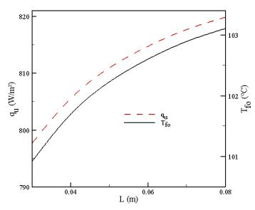
Figure 6.a: Variation of the useful flux and the outlet temperature as a function of the distance between the glass and the absorber at solar noon.
