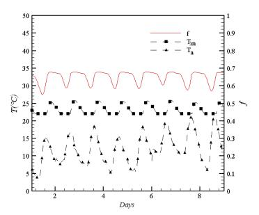
Figure 11: Internal building temperature  $T_{in}$  and liquid fraction f in a typical decade of January for the solar collector / PCM / concrete slab
