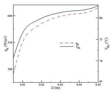
Figure 4.b: Variation of the useful flux and the outlet temperature as a function of the diameter of the tubes at solar noon.
