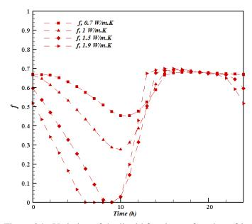
Figure 8.b: Variation of the liquid fraction as function of  $k_m$ .
