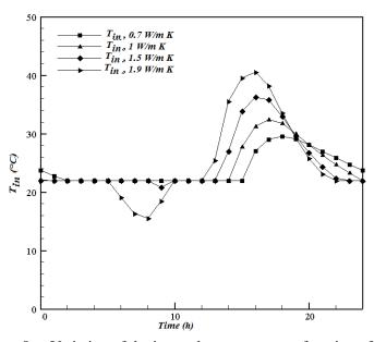
Figure 8.a: Variation of the internal temperature as function of  $k_m$ .
