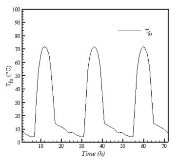
Figure 7.b: Typical outlet temperature of the solar collector during the month of January.
