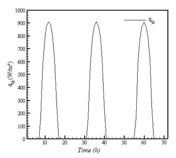
Figure 7.a: Typical useful flux of the solar collector during the month of January.
