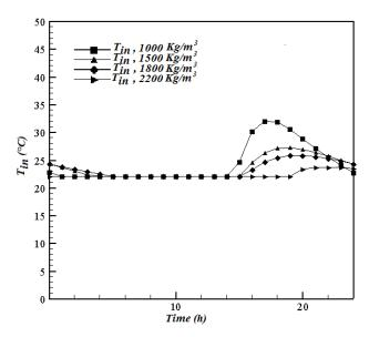
Figure 10.a: Variation of the internal temperature as function of  $\rho_m$ .
