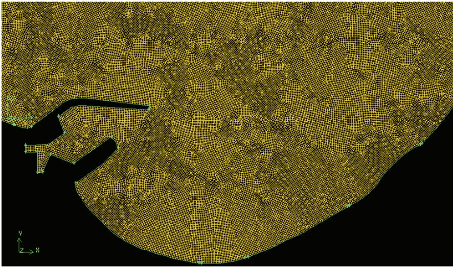
Figure 3: Detailed mesh of the free surface near the coast and estuaries of wadis
