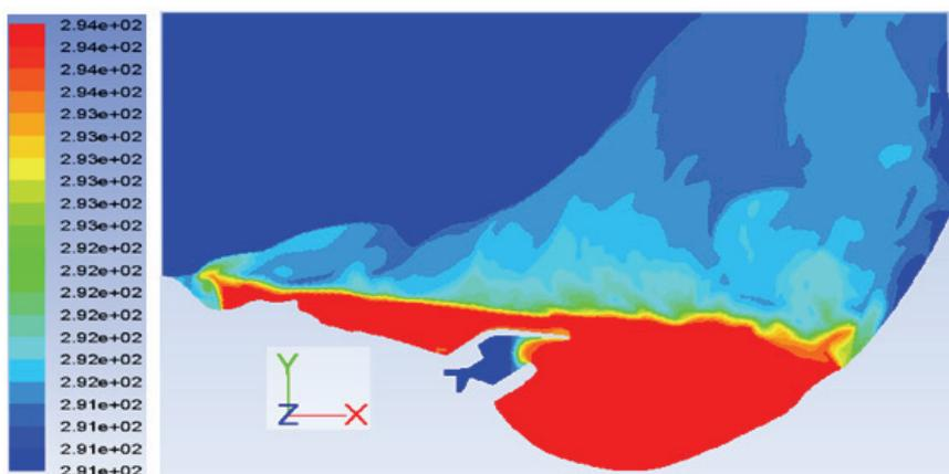
Figure 9: Temperature maps at the free surface of the bay after 24 hours
