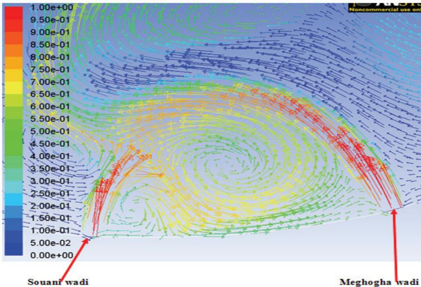
Figure 6: Velocity vectors colored by mass fraction of pollutant
