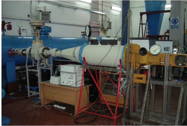
Figure 2: The supersonic blow-down wind tunnel.
