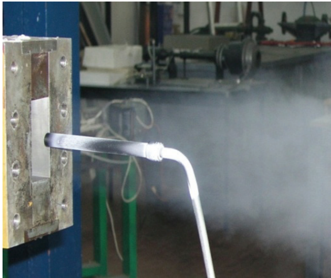
Figure 3: Condensation of residual humidity at the exit of the 2-D nozzle.
