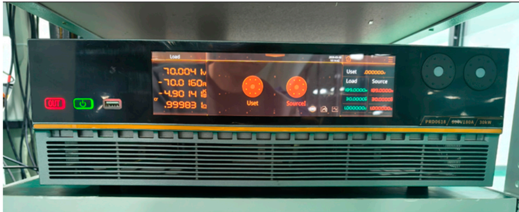
Figure 18: PRD0618 bidirectional programmable DC power supply simulates electrolyzer loads.
