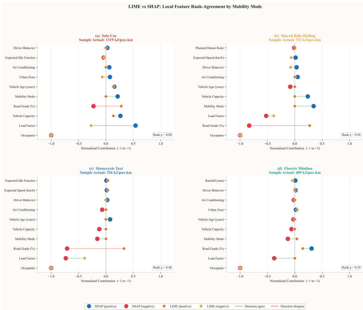
Figure 13: LIME vs. SHAP local feature rank-agreement for the median-residual trip in each mobility mode: (a) Solo Car; (b) Shared Ride-Hailing; (c) Motorcycle Taxi; and (d) Electric Minibus. The dumbbell plots show normalised feature contributions on a [-1, +1] scale. Green connectors indicate directional agreement between LIME and SHAP, whereas red connectors indicate sign disagreement. The corresponding Spearman rank correlation coefficient \rho is reported in each panel.
