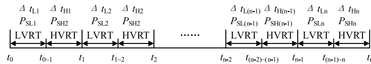
Figure 2: Schematic diagram of the -time L-HVRT process.
