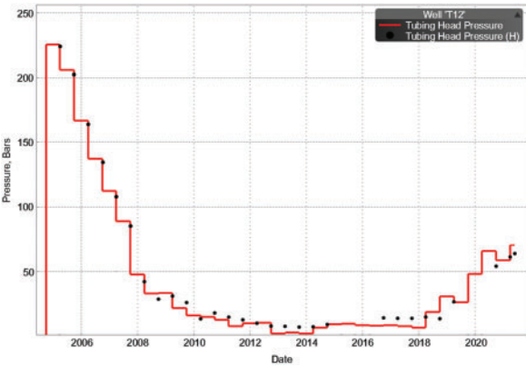
Figure 20: Wellhead pressure fitting diagram of well T12
