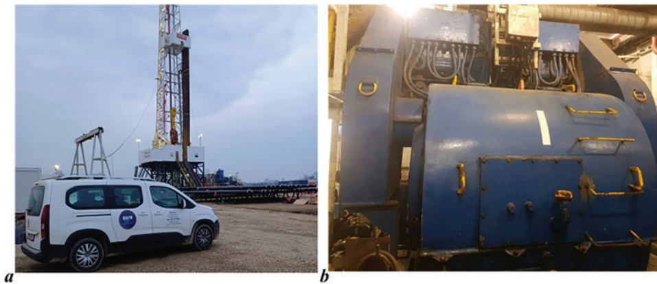
Figure 13: Photographs of a deep drilling rig (a) and mud pump drive (b)
