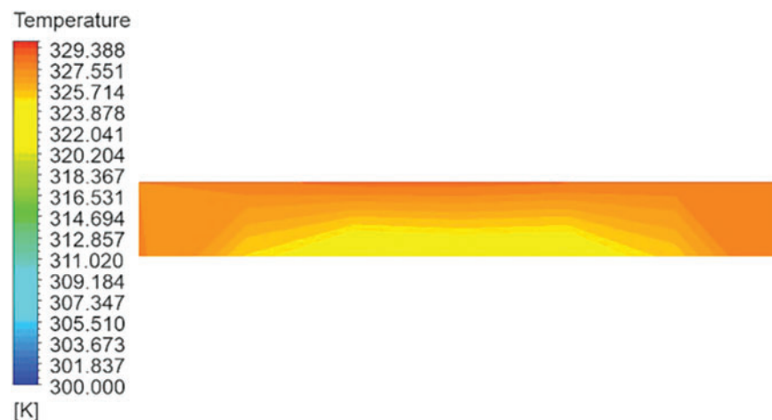
Figure 11: Distribution of temperature in a nano encapsulated phase transition material with a 5 wt.% fraction
