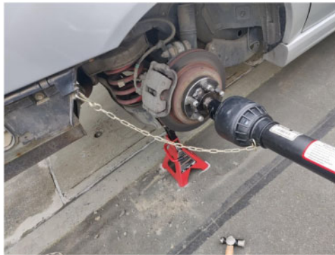
Figure 4: Hub spline adapter mounted to PTO shaft for connecting vehicle's driving wheel to external machinery
