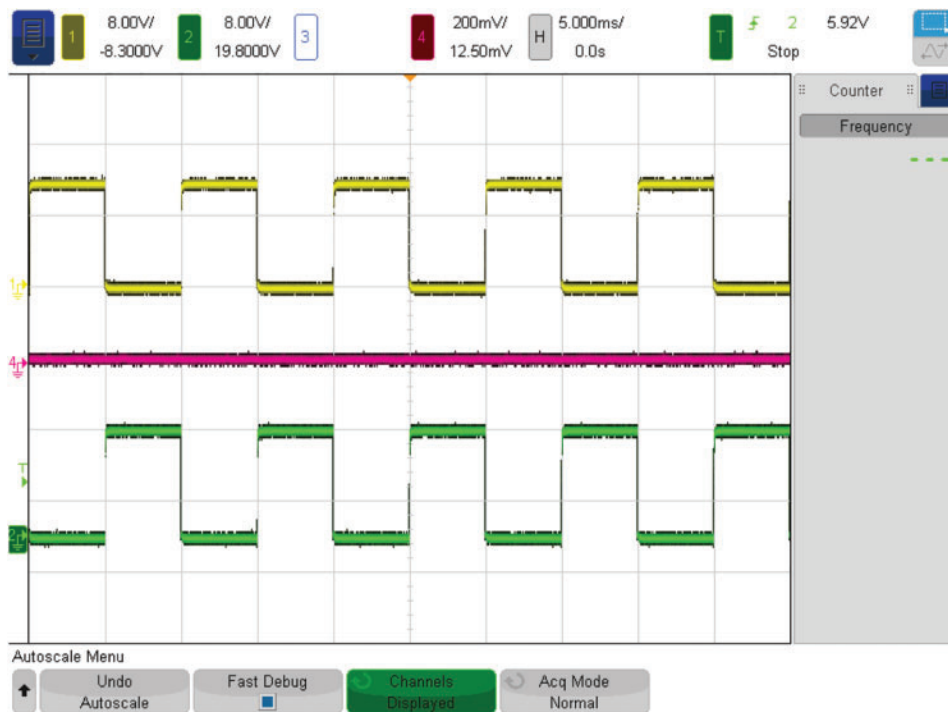
Figure 15: Comparison of output PWM waveform of three-cell equalization circuit amplification module and MCU
