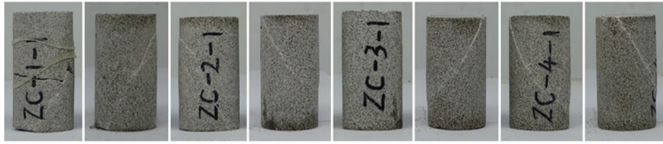
Figure 2: Failure mode of rock sample
