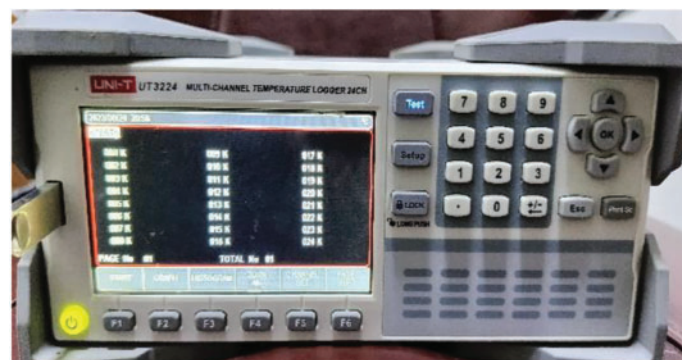
(a) Temperature data logger with 24 channels (Uni-T UT 3224 model)
