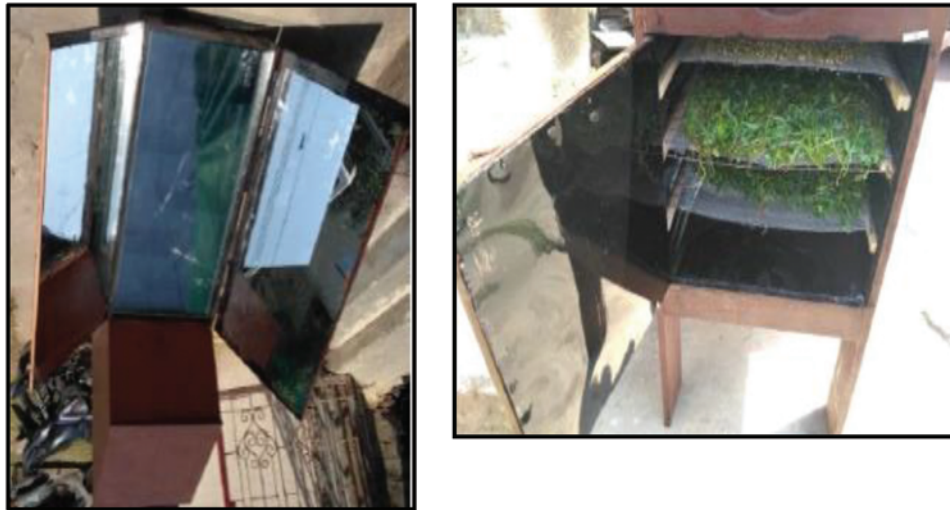
Figure 15: Reflecting mirror and insulating chamber of indirect dryer. Adapted from Gupta et al. [40]
