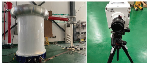
(b) Voltage generation system (left) and high-speed camera (right)
