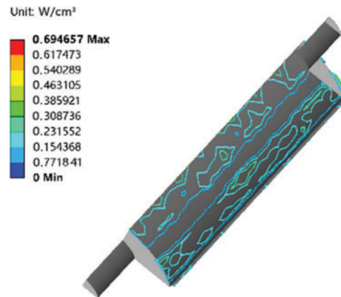
Figure 11: Cloud diagram of the eddy current loss density of a permanent magnet
