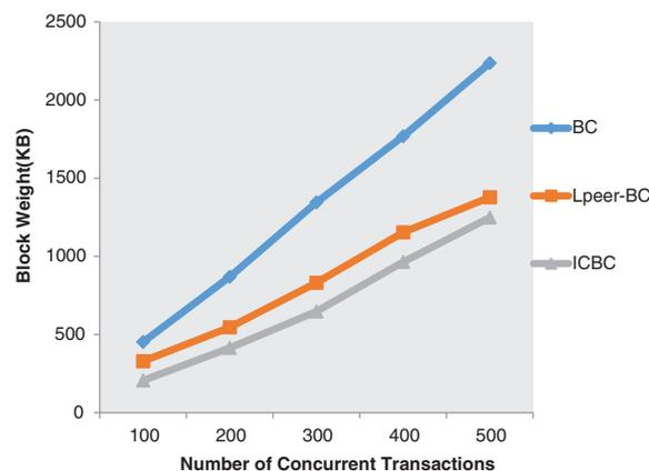
**Figure 3:** Block weight for concurrent application transactions
