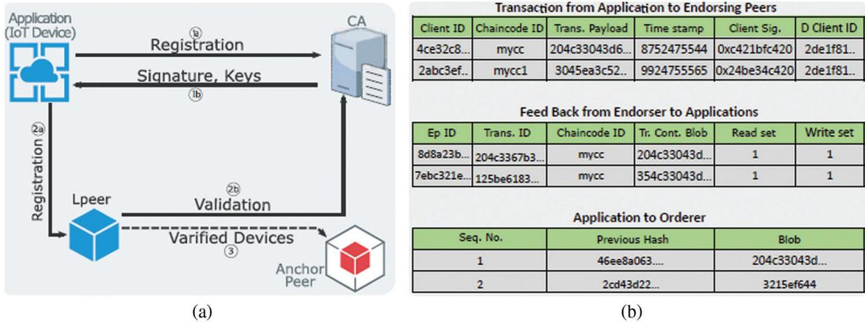
**Figure 2:** (a) Device registrations in IoTs, (b) Hyperledger's generic transaction format
