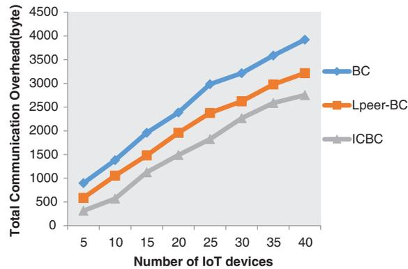
**Figure 6:** Impact of communication overhead vs. block chain approaches
