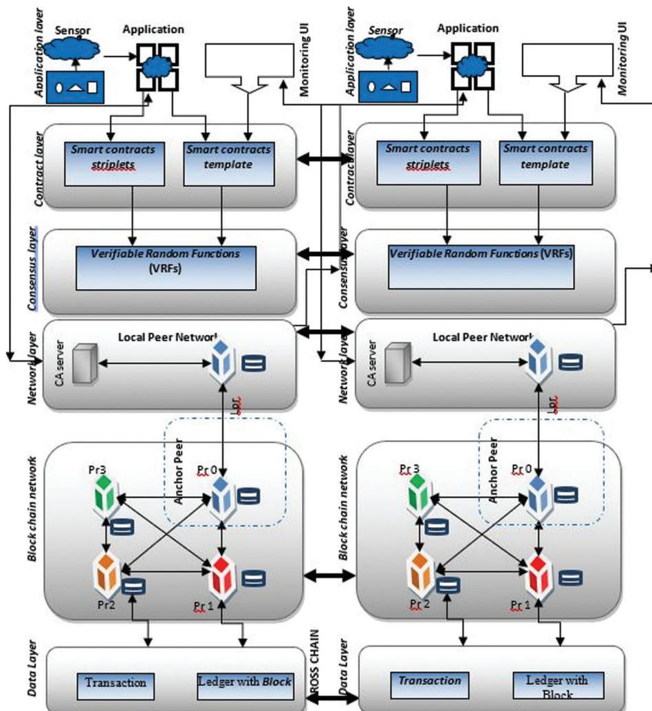
Figure 1: Proposed icbc framework with a local peer-based network model
