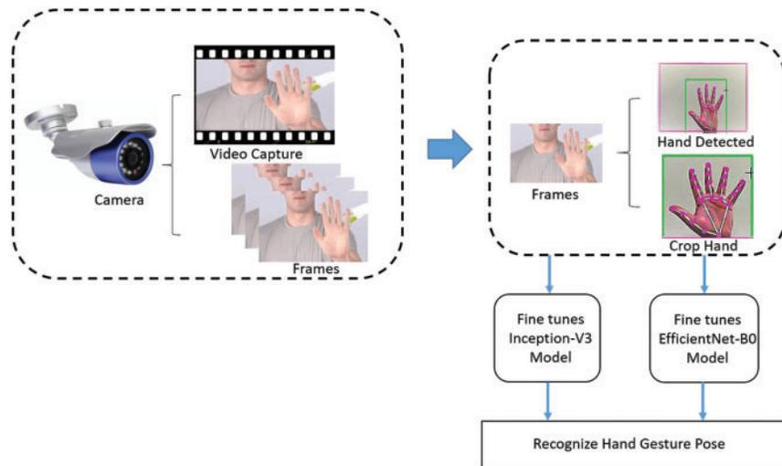
**Figure 8:** Real-time hand gestures recognition framework
