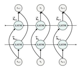
Figure 2: Structure of BiLSTM
