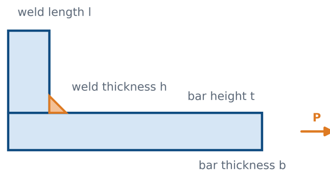
Figure 10: Unified schematic of the welded beam design problem.
