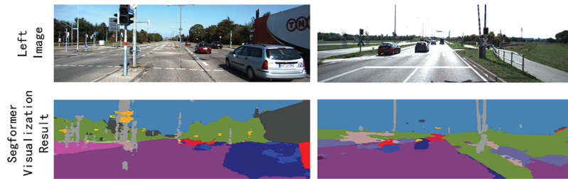
Figure 2: A visual example of SegFormer extracted semantic features
