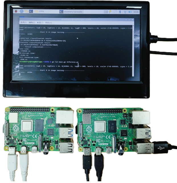
Figure 5: EPPA implemented with the Raspberry Pi (as a resource-limited device)
