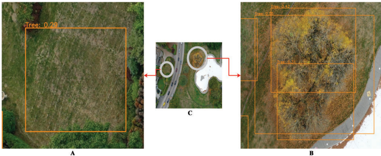
Figure 7: “A” represents the grass area mistakenly detected as a tree, while “B” represents a single tree incorrectly detected as multiple trees by YOLOv9s, “C” is the tested sample
