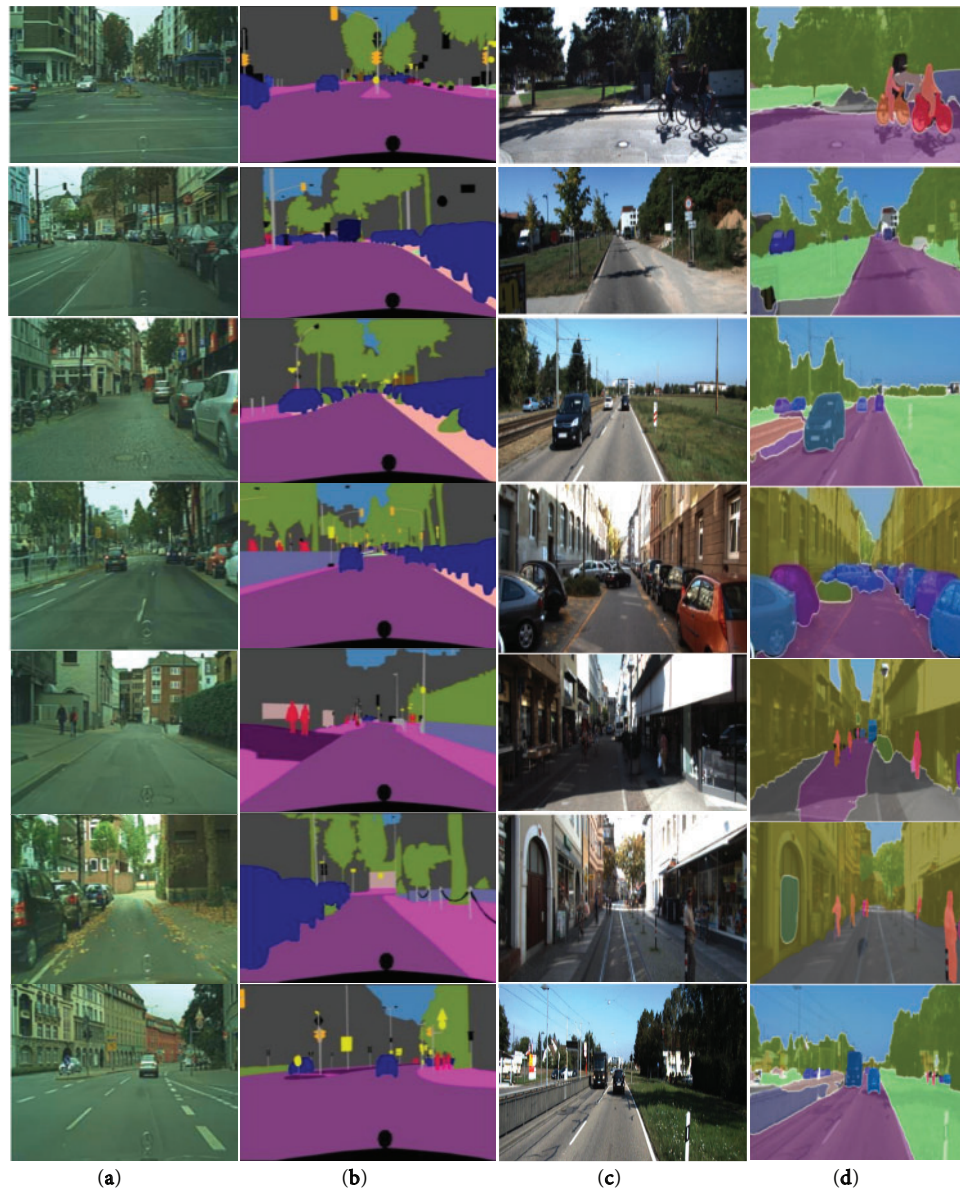
Figure 6: Panoptic segmentation performance of the recommended network can be seen using two validation datasets: (a) input image for Cityscapes; (b) suggested output for Cityscapes; (c) input image for KITTI; and (d) proposed output for KITTI
