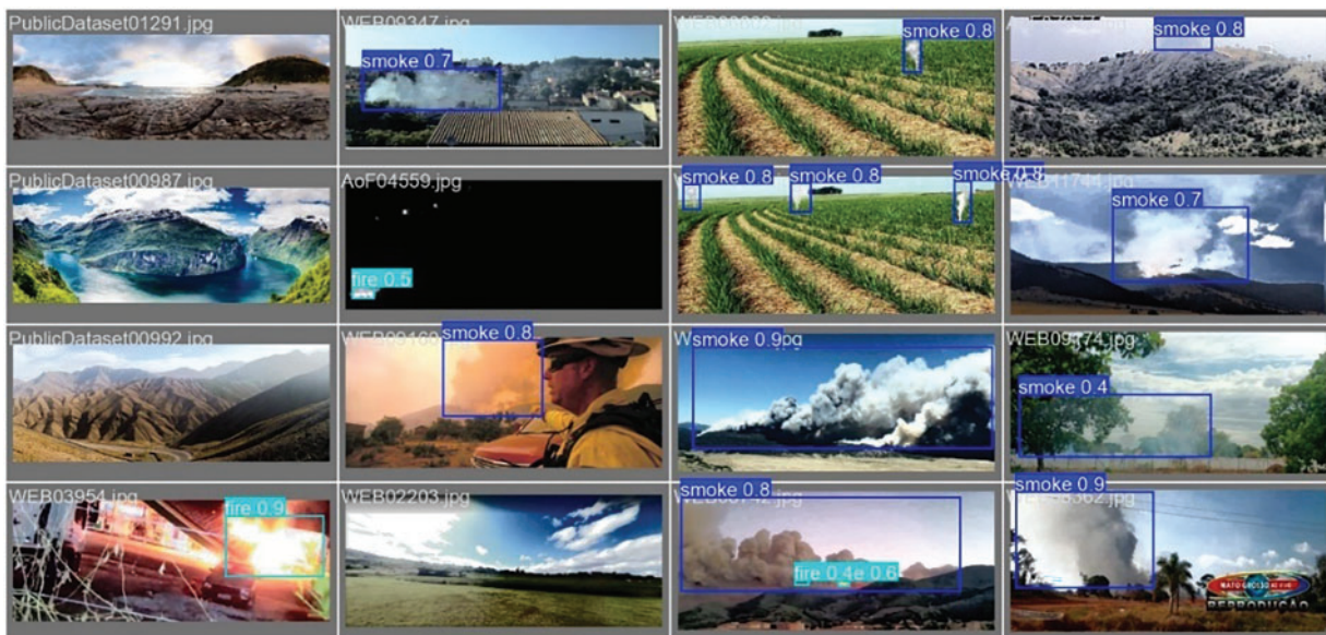
Figure 7: Validation Batch 0 with YOLOv11x and X Dataset (HE)
