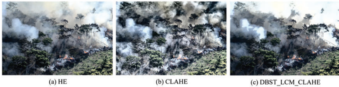
Figure 2: Examples of image enhancement methods with (a) HE, (b) CLAHE, and (c) DBST-LCM CLAHE
