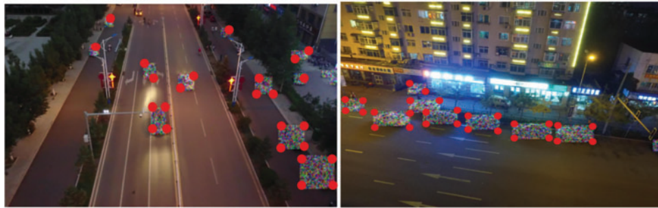
Figure 6: Dense-SIFT feature extraction, grid-based keypoint sampling (colorful dots) over a vehicle ROI
