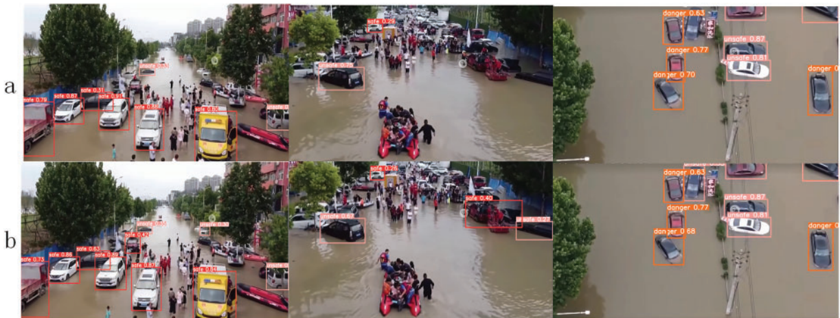
Figure 8: Experimental visualisation results. (a) demonstrates the object detection performance of the base YOLOv9 model. (b) presents the de-tectio effect of the improved method proposed in this paper
